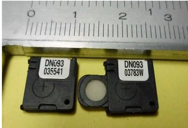
FIG. 3.2. Detectores Nanodot OSL ( $Al_2O_3:C$ ) Landauer INC.
